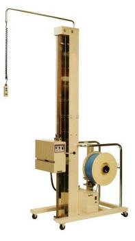
The GRB200 is a semi-automatic horizontal strapping machine for pallets. It is easy to positioning the plastic strap by means of a folding arm. The launching, tensioning and sealing of the plastic strap is activated by a remote control.
